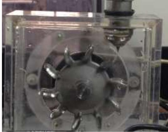
**Figura 1:** Turbina Pelton AMRFIELD FM-32 [13].
