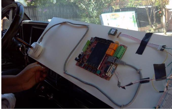
**Figure 11** - VIRMS Remote Client device board.
