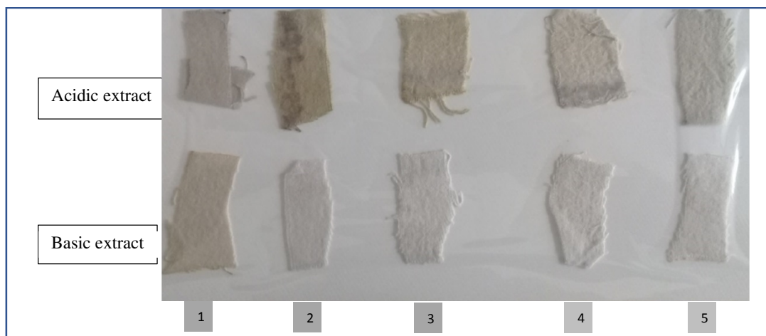
Figure 2: Results of the dyeing control process done on the cotton fabric tinted with the acidic and basic extracts of Brachyotum microdon (flowers). 1 Fabric rinsed with water; 2 Fabric washed and rubbed with water; 3 Fabric washed with a detergent and then rinsed (without rubbing); 4 Fabric washed with a basic detergent and rinsed (with rubbing); 5 Fabric washed with an acidic detergent and rinsed (with rubbing).
