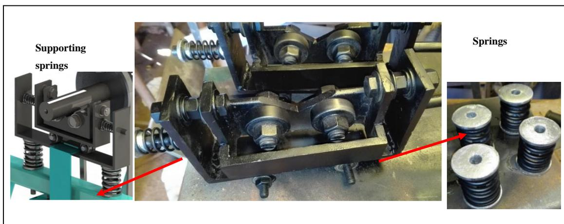
Figure 11: Suspension prototype for rotor balancing measurement system.
