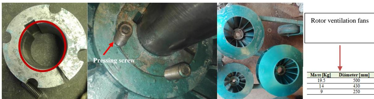
Figure 28: The rotor ventilation fans and the adjusting system with the pressing screw.
