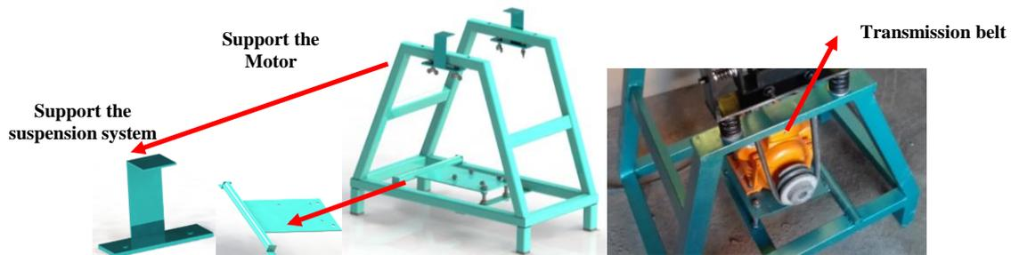
Figure 10: Designed bench machine, drawing in Solidworks.
