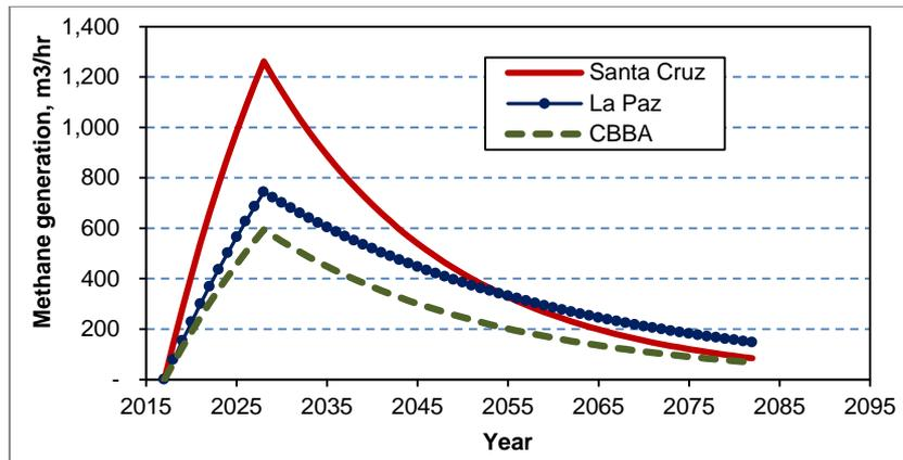
**Figure 3 - Methane generation obtained from the landfill.**
